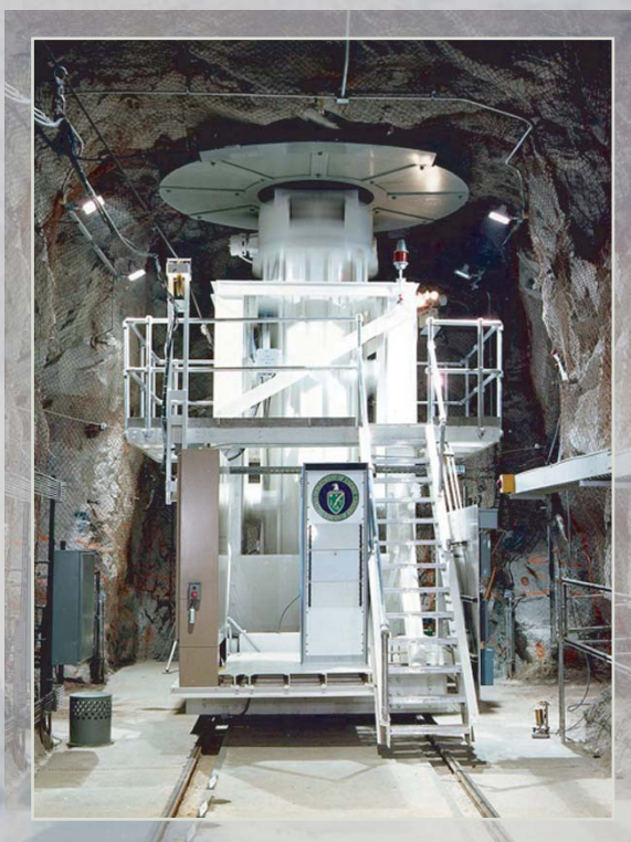
Remote Emplacement Vehicle, Spent Fuel Test, Climax Mine, Area 15, 1985
