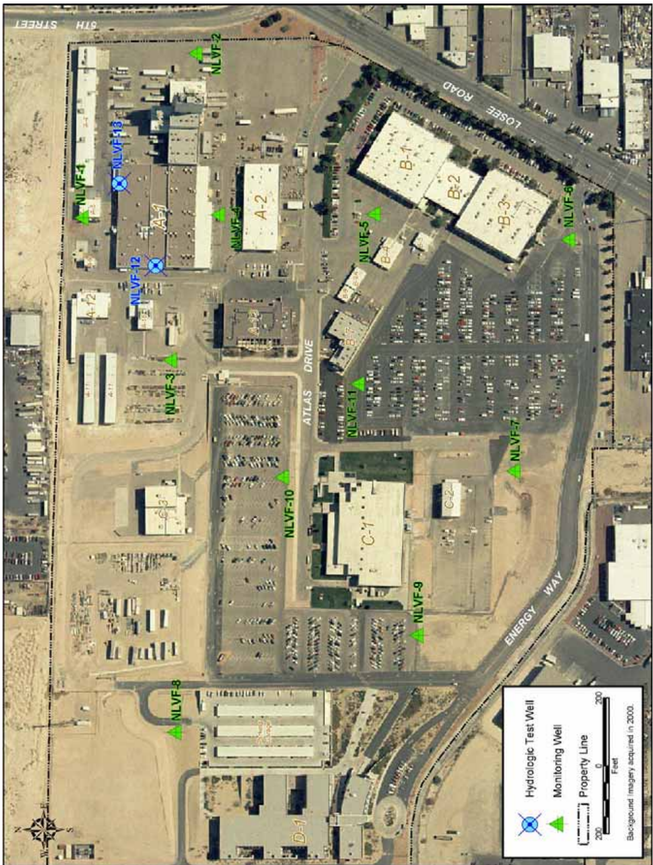
Figure B-2. Monitoring wells and hydrologic test wells constructed at NLVF
